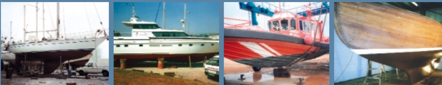
Coppercoat can be applied to craft of virtually all materials, including left to right: GRP fibreglass (1994), steel (1994), aluminium (1994), wood (1992)
